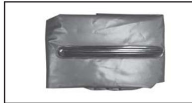
5e. Fold kayak in half, with strake up, as shown in the above image.
