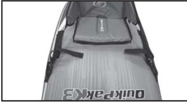
15. Connect seat backrest buckles to buckles on kayak.
