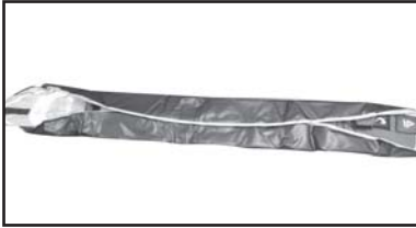
5b. Fold kayak lengthwise again, as shown in the above image.
