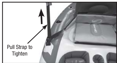
17. Adjust seat back straps to your desired tension.
